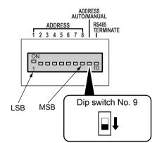
(2) Use dip switch Nos. 1 to 8 to set the least significant byte of the IP address as a binary number.
